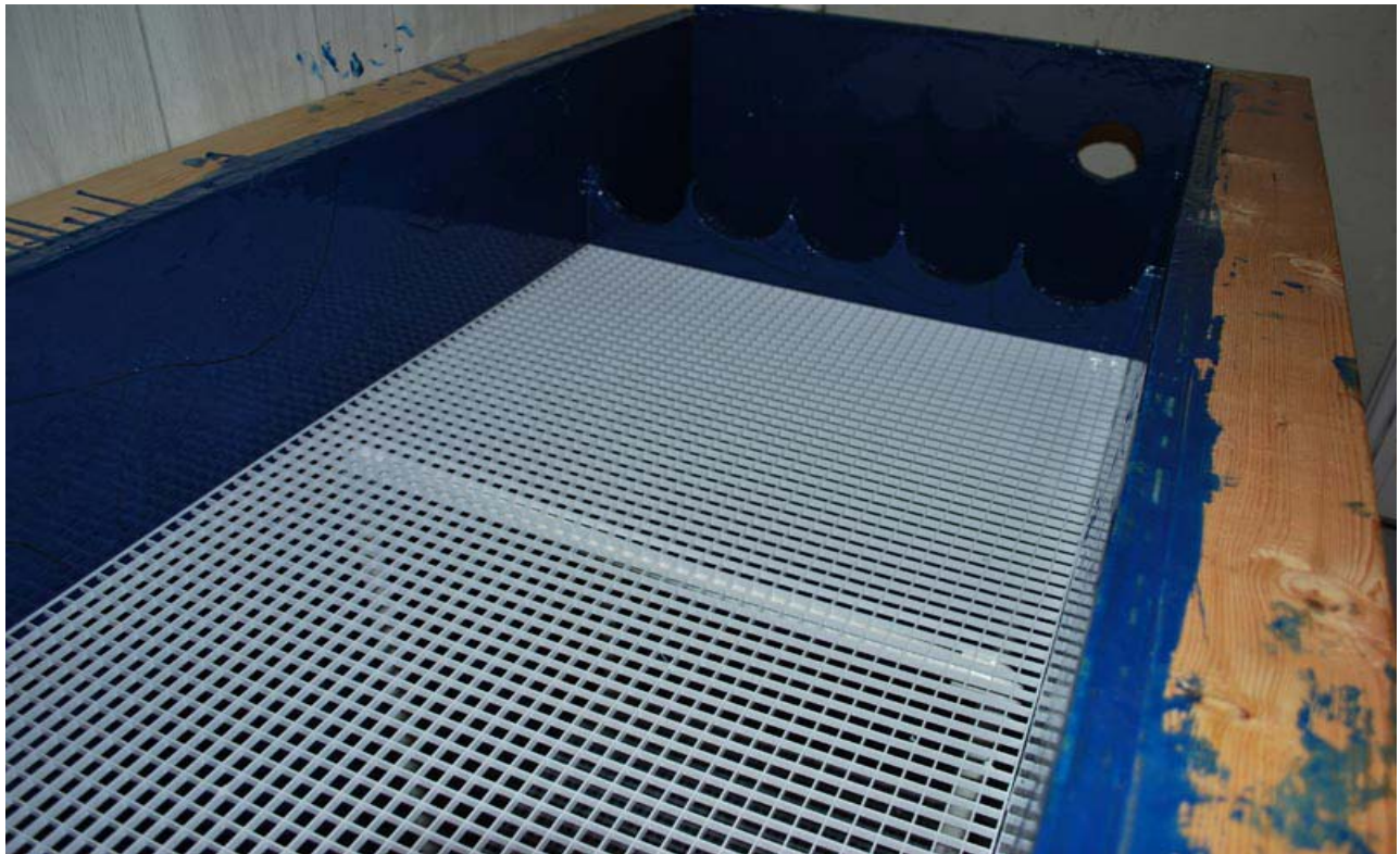
Top of bio media chamber that will support the mechanical filter pads.
