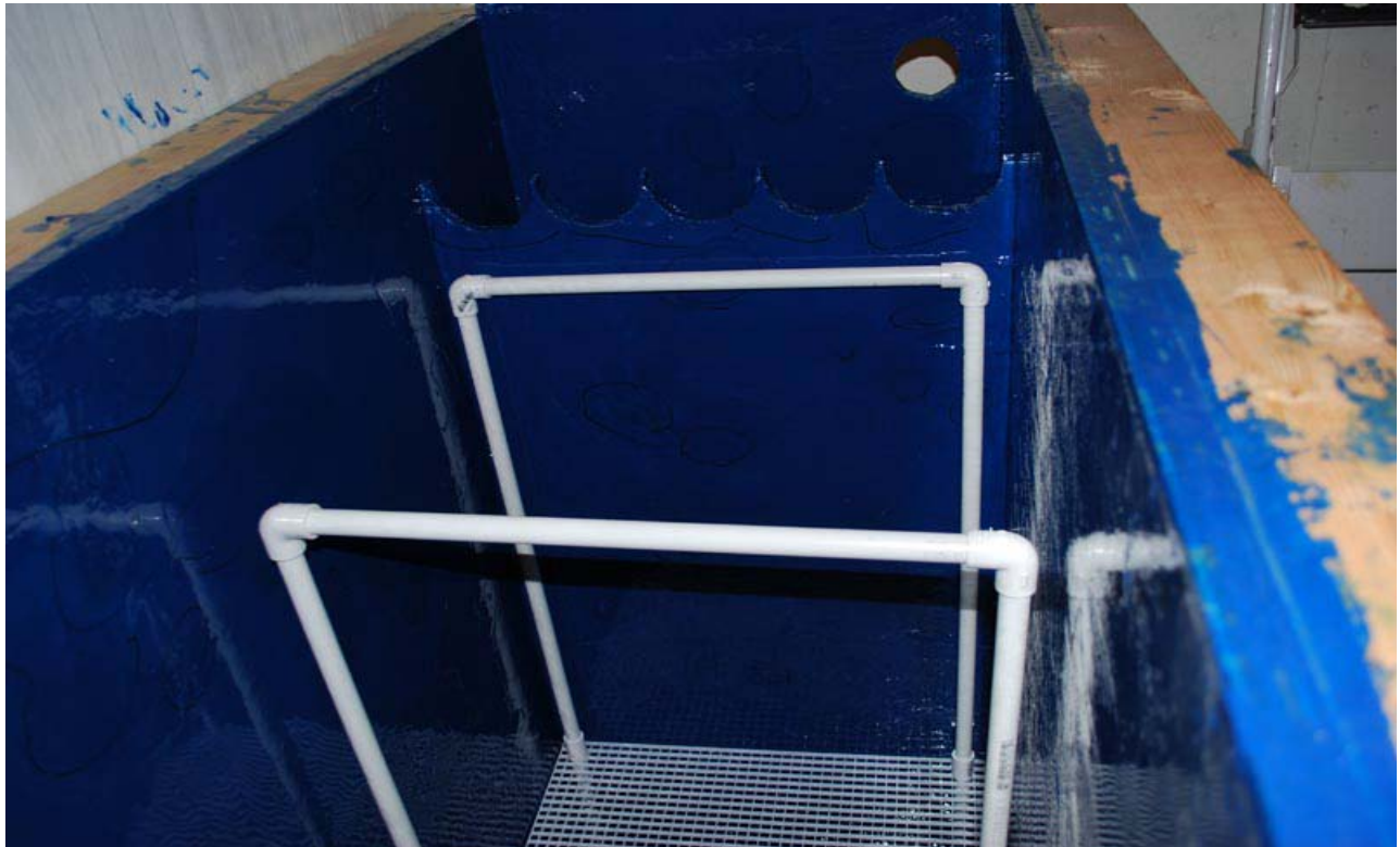
Top of bio media chamber that will support the mechanical filter pads.
